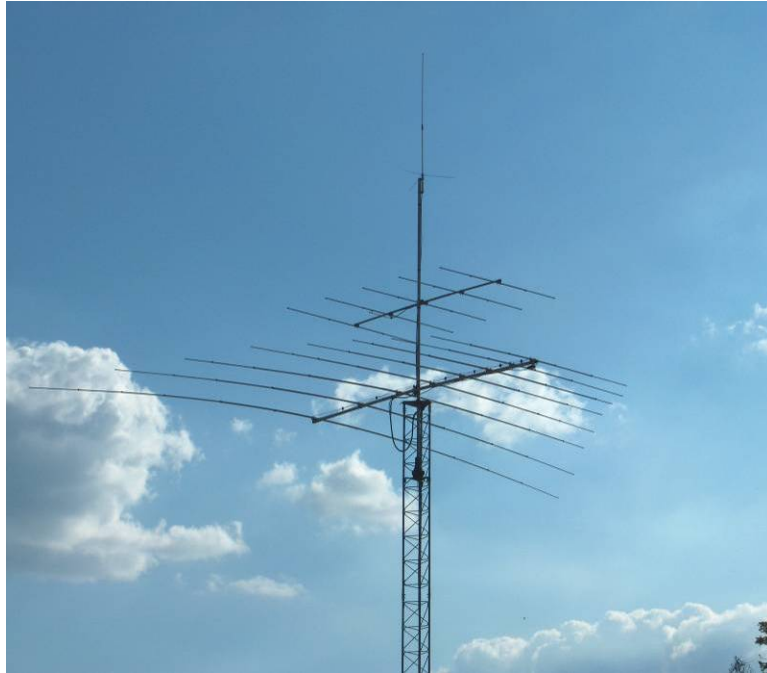
Figure 60 - Club Station Equipment for the San Antonio Radio Club W5SC. On top is a dual band vertical for 2 meters and 70 centimeters. The next antenna down is a horizontal 6 meter 5 element Yagi type beam and on the bottom is a HF Log Periodic Beam. Photo by N5IUT
