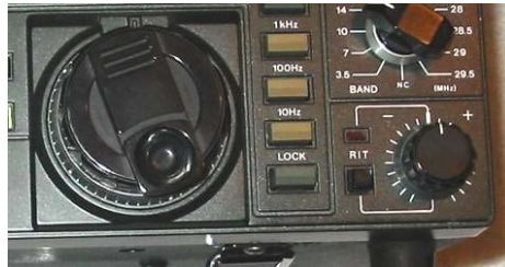
Figure 36 - The small knob on the right adjusts the RIT when the RIT button beside it is activated. Photo by K3DIO
